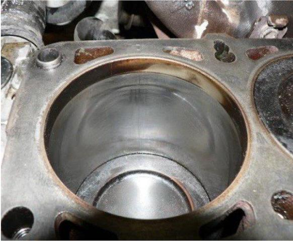
*Bore glazing – Blue Chip Lubricants pic*
